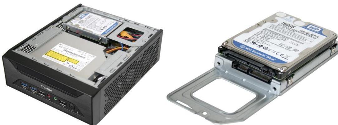
The Shuttle XPC slim Barebone XH110 supports one optical drive in 5.25" slimline format and two 2.5" drives (e.g. 2.5" hard disk and 2.5" SSD). A second 2.5" drive requires an additional SATA cable and mounting screws which are not included. The storage drives (hard disk and optical drive) are not included in the delivery of the XH110. **Notice:** For high ambient temperatures over 40°C we strongly recommend to use SSDs instead of hard disk drives.
