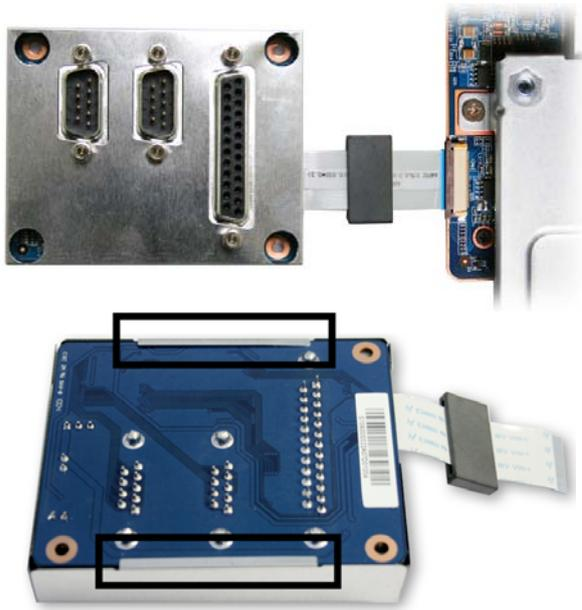
**(10)** Mount the electromagnetic shield of the COM/LPT adapter for which the hexagon screws need to be removed temporarily. Note: The electromagnetic shield must be attached to board so that the metal fixations of the shield clasp the board. Please connect the adapter with the mainboard afterwards. Make sure to have the cable and ferrite core aligned properly so that the electromagnetic shield is not damaged during further assembly.
