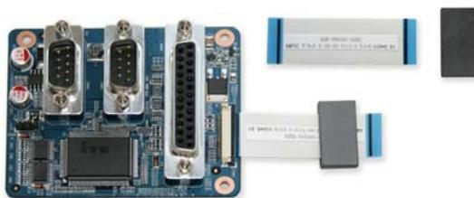
**(9)** Optionally a COM/LPT adapter (PCL68) can be installed. This adapter is to be connected to the mainboard via a ribbon cable. The connectors of the ribbon cable have one securing clip each that needs to be pushed forward first. Having then connected the ribbon cable to the mainboard, the cable is to be fixed with the securing clip with the contacts of the cable facing towards the board. Please do not forget to lead the cable through the ferrite core.
