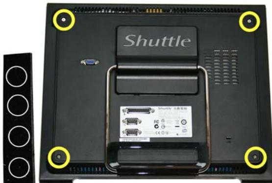
**(12)** Replace the existing type plate sticker by the sticker as delivered to provide openings for the COM/LPT ports. Please re-mount the case cover and the stand vice versa. Finally, click the cap with the Shuttle logo back into place and cover the four screw holes with the self-adhesive rubber coverings included in the delivery scope.
