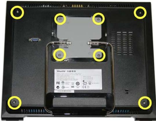
**(3)** Loosen the four cross-head screws (or Phillips screws) to remove the stand. Remove the four cross-head screws that fix the case cover.
