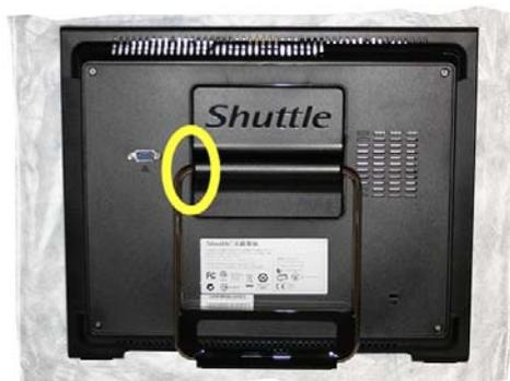
**(2)** Disconnect the device from the mains and put it on a soft base with the display facing downward and fold the stand vertically upward. Next, carefully remove the cap with the Shuttle logo that is clicked into place by six hooks. The cap can be loosened using a plastic card.
