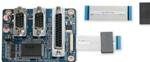
**(9)** Optionally a COM/LPT adapter can be installed. This adapter is to be connected to the mainboard via a ribbon cable. The connectors of the ribbon cable have one securing clip each that needs to be pushed forward first. Having then connected the ribbon cable to the mainboard, the cable is to be fixed with the securing clip with the contacts of the cable facing towards the board. Please do not forget to lead the cable through the ferrite core.
