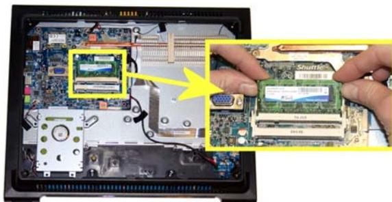
**(8)** Now install the memory modules and make sure they are clicked into place properly. Please see the notch when installing the module to make sure it faces in the right direction.
