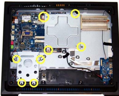
**(6)** Another shielding is fixed by four screws. Only remove this part to install or exchange memory modules. Loosen the four screws of the drive cage and remove the latter.
