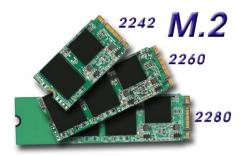
The M.2 slot (type 2280) is fully-equipped with 4X PCI-Express v3.0 lanes and SATA 3.0 interfaces. Modern M.2 SSDs with PCI Express interface (PCIe) provide a significant higher bandwith compared to the usual SATA standard. Type 2280 means it supports the usual M.2 cards with a width of 22mm and a length of 80mm, but also 2242 and 2260 standard cards are supported.
