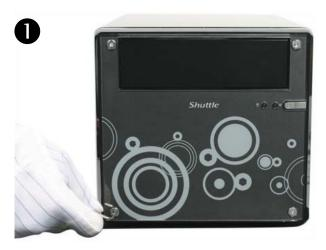
Unfasten the front panel by removing the four screws. Remove both the transparent glass and the image.
