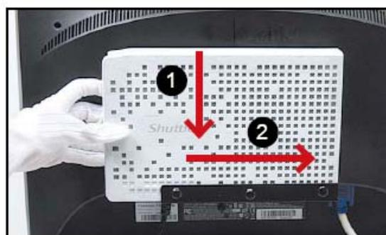
As shown, install the XS35 in the VESA MOUNT and push it towards the direction as indicated by the red arrow.
