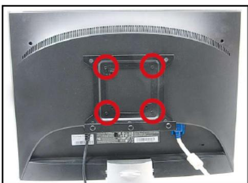
Fasten the VESA MOUNT at rear of LCD monitor with four screws.
