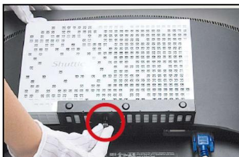
Check that it is properly aligned, then tighten securely with one thumbscrew.
