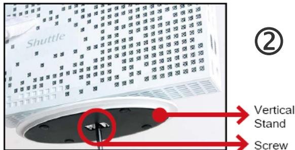
Unscrew one screw of the stand mount and remove the vertical stand.
