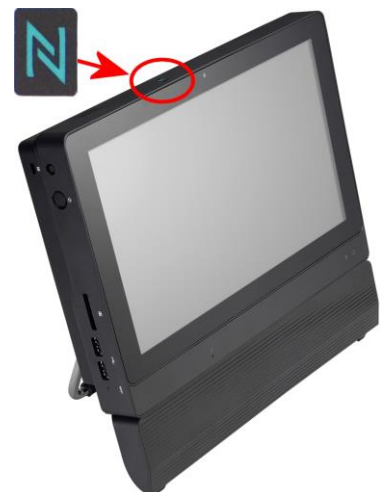
The sticker with the NFC icon marks the position of the NFC antenna inside the Shuttle XPC All-inOne Barebone P20U.
