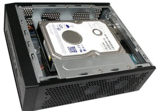
Shuttle Slim-PC Barebone (3 litres) with built-in Accessory PHD4 including 3.5" hard disk drive.
