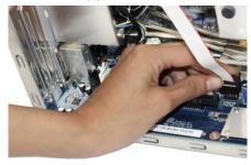
8 Make sure that the marked lead of the ribbon cable and the marking on the mainboard are on the same side.
