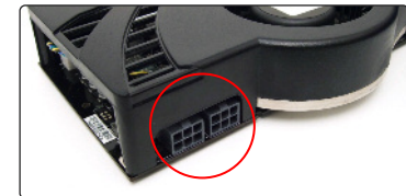
Graphics card with two 6-pin power connectors
